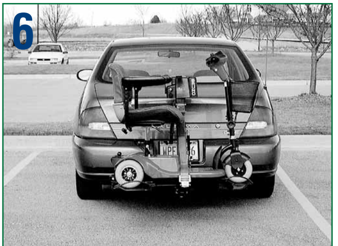
6 Lower lever, secure belt to Velcro®*, turn key to OFF and remove key.
