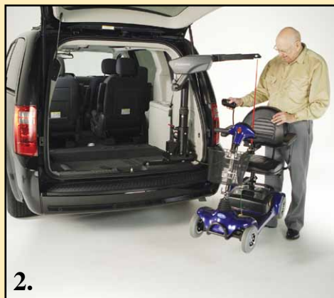
2. Raise mobility device by pressing button...
