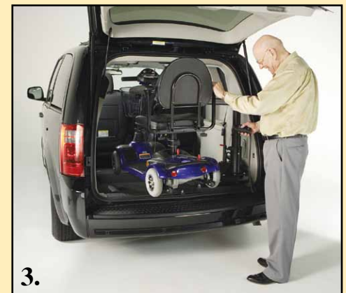
3. Manually rotate mobility device into vehicle.
